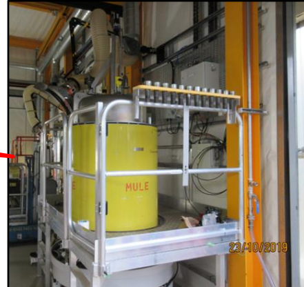
Photo of a MOSAIK ® DCIC in its filling station
