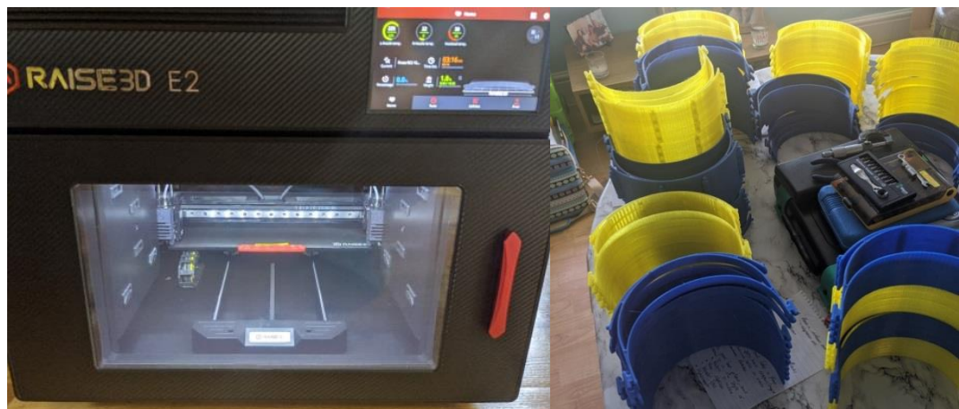
The new 3D printer at Coleg Meirion Dwyfor producing the visors
