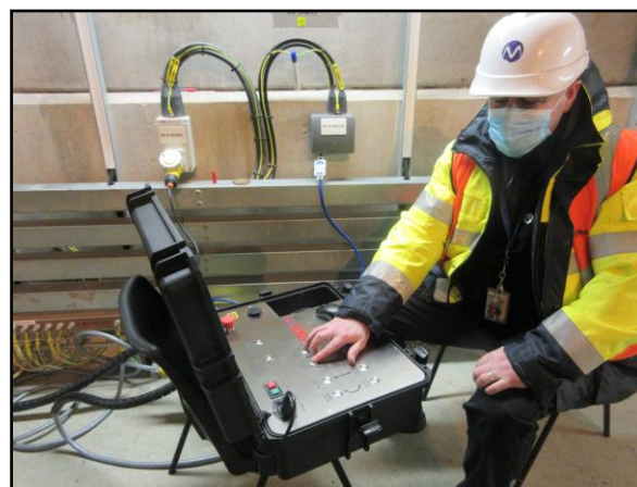
Dumper Bot during operator training within clean conditions prior to being deployed to the WILWREP inner tent.
