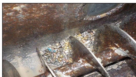
Typical debris collected within worm drive casing
