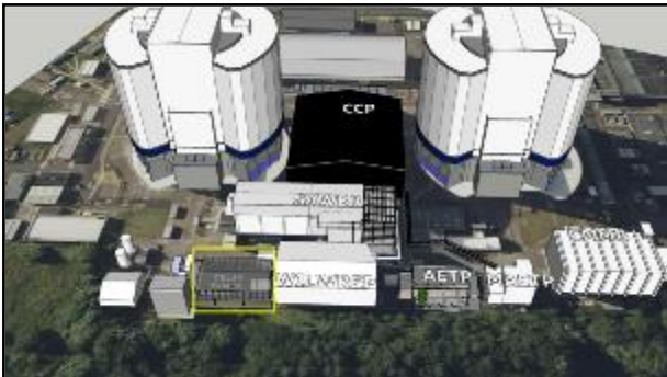
3D Model showing location and configuration of delay tanks (highlighted in yellow)
