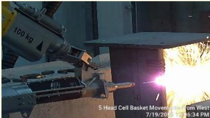
Remotely-operated laser cutting trials within the Head Cell
