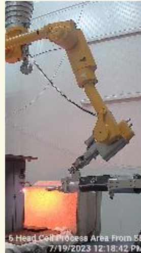
Remotely-operated laser cutting trials within the Head Cell
