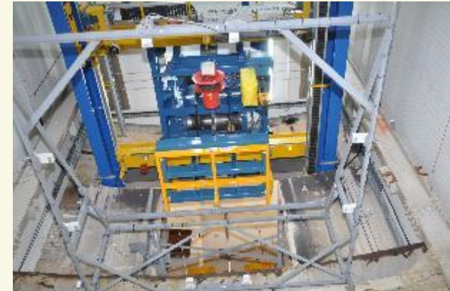
Testing of the Intermediate level Waste "Bin" Assay Array
