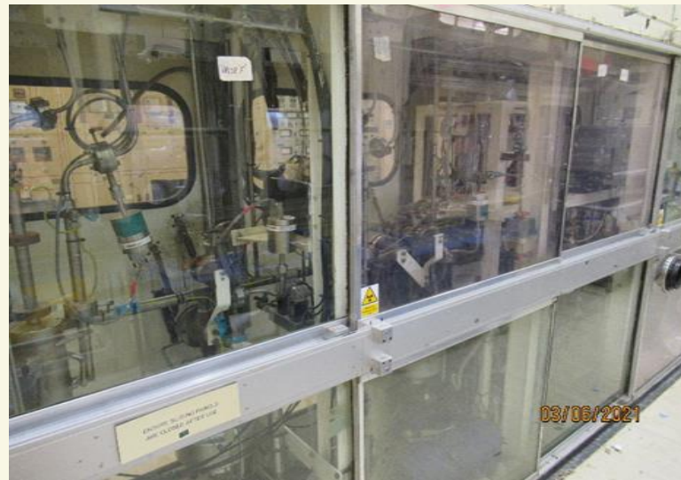
Contaminated Tritium Purification Vessels and Pumping Systems Within the Process Cubicle
