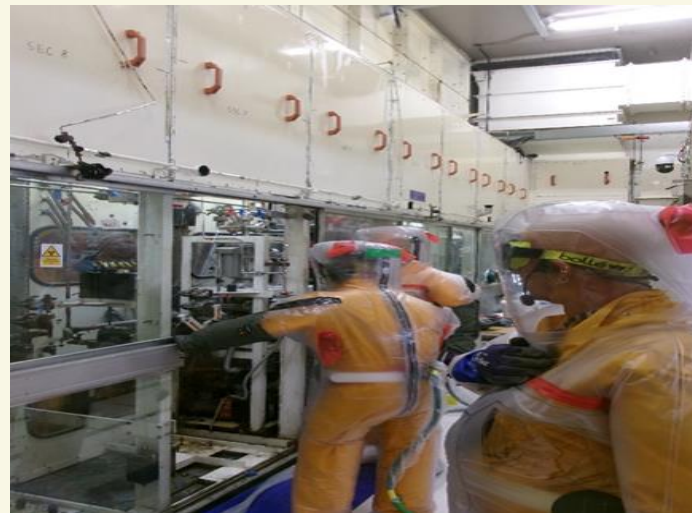
'Crimp & Cut' and ILW Retrieval Operations Within the Process Cubicle
