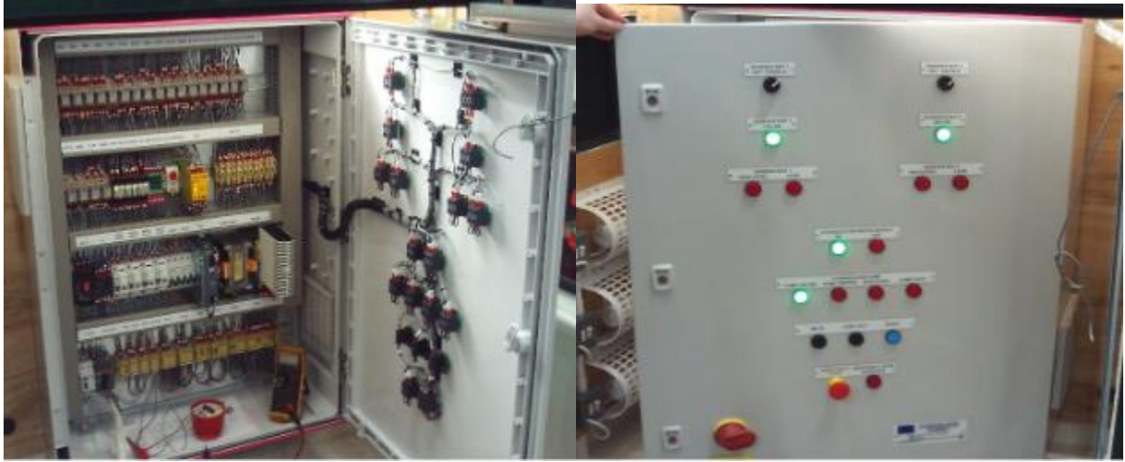
Factory Acceptance Test photos showing weatherproof electrical enclosure and control unit.
