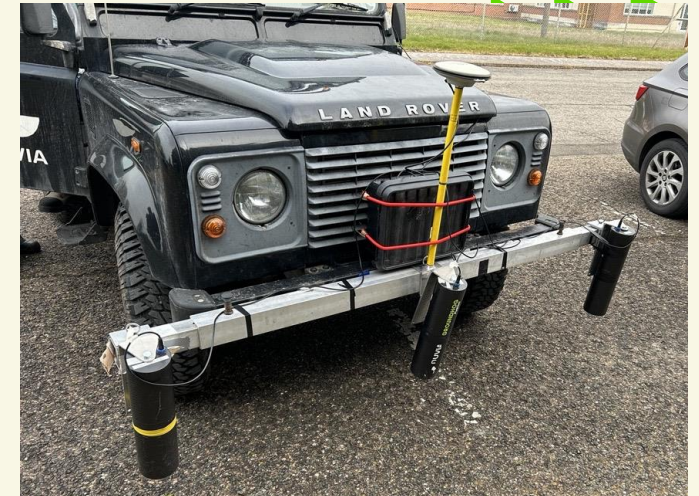
Nuvia's 4x4-mounted GroundHog Gamma Radiation Survey Equipment during the B540/551 Area surveys
