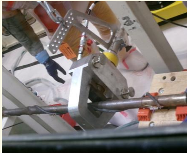
‘Crimp & Cut’ methods used to reduce tritium discharge and retain column packing materials
